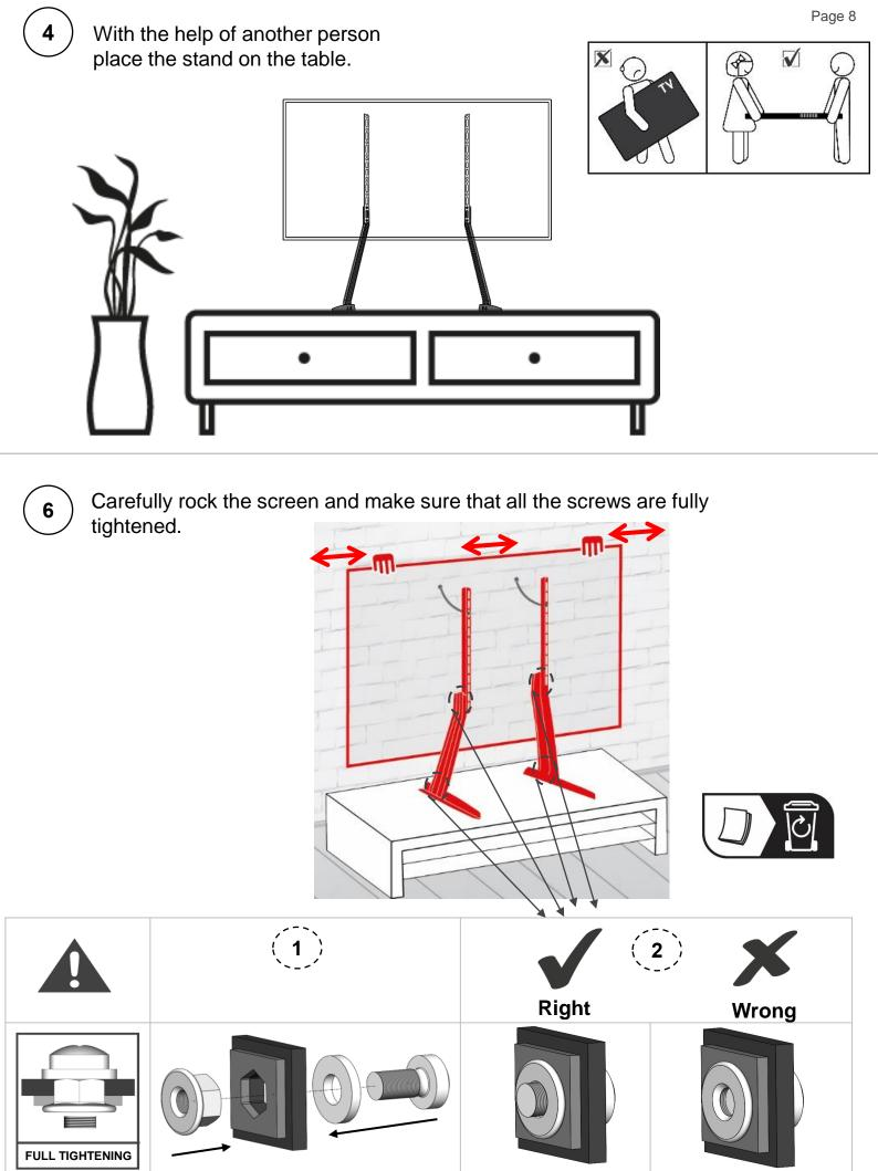
**Full Tightening** — Whenever the full tightening icon is displayed, make sure to place a nut inside the hexagonal slot and that the endpoint of the screw crosses the edge of the nut.
